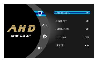
Main menu: Brightness/ Contrast /Saturation/ Auto Brightness/Reset setting.Press "AV" button to select up and down.
