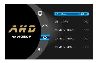
System: Language/ Picture UP and DOWN / CAM1,CAM2,CAM3 mirror image setting
