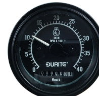
0-523-78 | 12/24V 86mm Ø Tachometer 270° dial, 0-4,000rpm. Programmable for alternator pick-up
